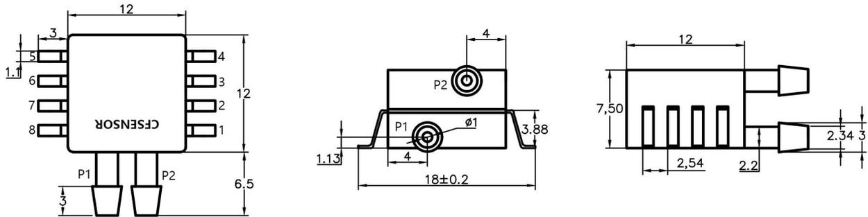
Note: Port 1(P1) as High pressure cavity, and Port 2(P2) as Low pressure cavity.
